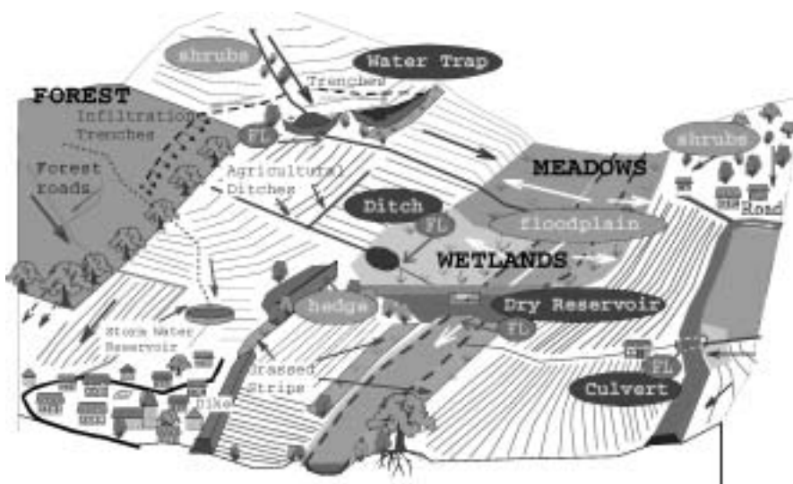
Figure 1 Opportunities for slowing down (light tags) or temporary storage (dark tags) using flow limitation (“FL” tags) in a catchment.
